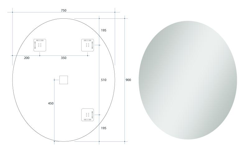
Note: All dimensions are in millimetres (mm)
