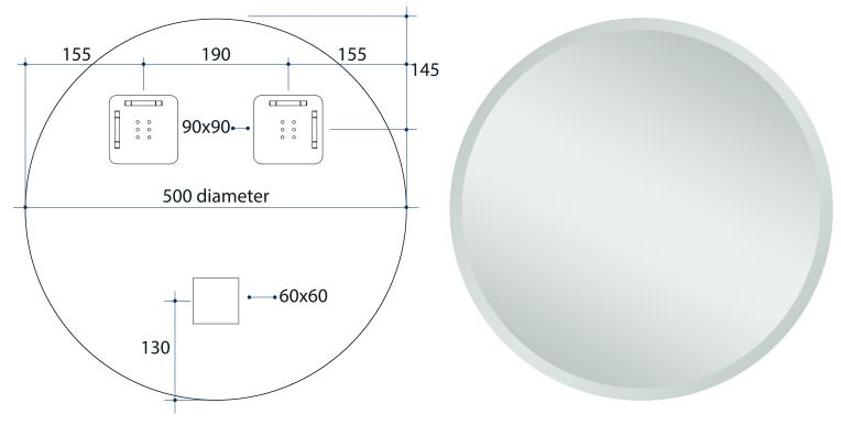
Note: All dimensions are in millimetres (mm)
