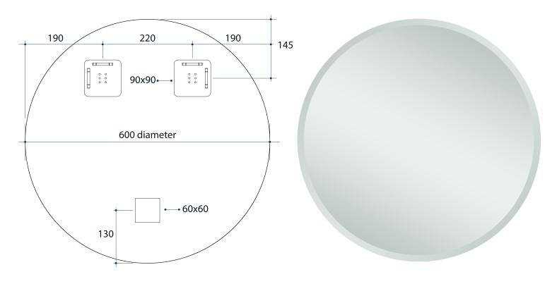
Note: All dimensions are in millimetres (mm)
