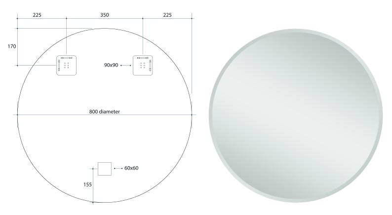
Note: All dimensions are in millimetres (mm)
