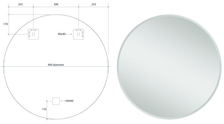
Note: All dimensions are in millimetres (mm)
