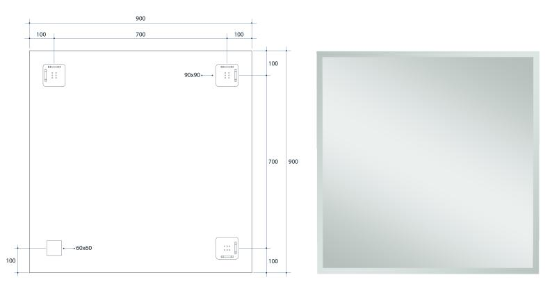
Note: All dimensions are in millimetres (mm)
