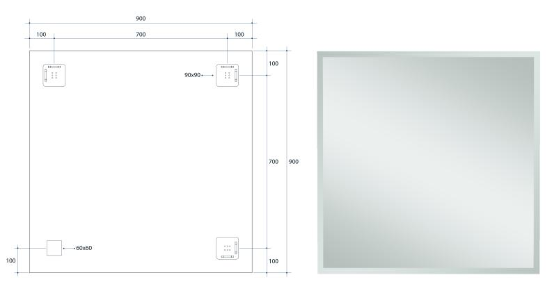
Note: All dimensions are in millimetres (mm)
