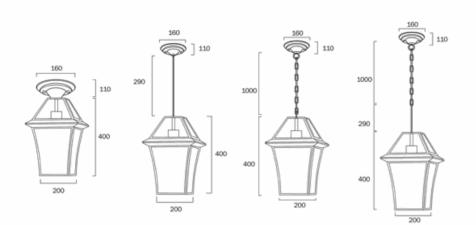
All representations within this document are subject to copyright. ELECTRICAL INSTALLATIONS MUST BE PERFORMED BY A QUALIFIED ELECTRICAL CONTRACTOR AND INSTALLED IN ACCORDANCE WITH AS/NZS 3000. NOTE : All images , descriptions and dimensions are indicative. Please check latest version of item detail on Telbix website prior to ordering or installation.
