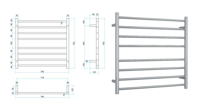
This rail has Multiflex wiring which means that there is a connection point on both the left and right hand side of the rail and the lead can be connected to either side. Being a dry electric element rail, this can be mounted either way up meaning the wiring can be from any of the four mounting points.
